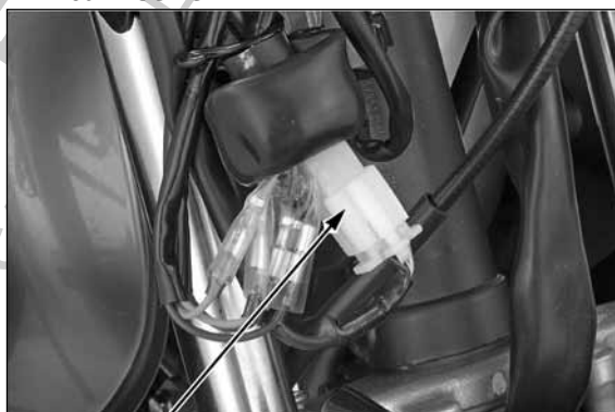
NXR150 ESD: CONECTOR 6P (NATURAL) NXR150 ES: CONECTOR 3P (NATURAL) NXR150 KS: CONECTOR 2P (NATURAL)
